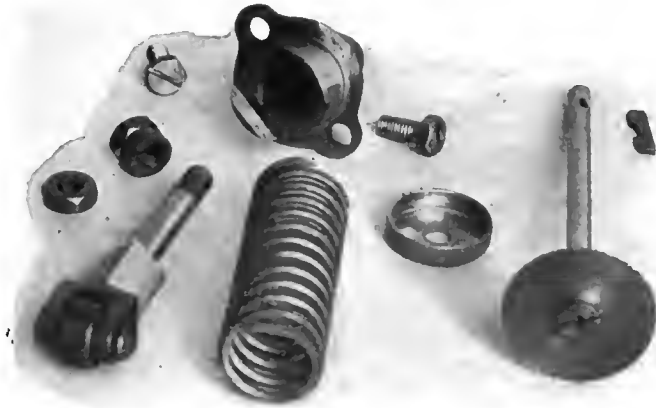
PARTS OF LOCOMOBILE VALVE SEPARATED, SHOWING PUSH-ROD AND GUIDE, SPRING AND STEM WITH MUSHROOM.
